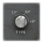
The TYPE switch allows selection of the type of filter to be used. HP selects High-pass, BP selects Band-pass and LP selects Low-pass. A High pass filter passes through frequencies above the cutoff, and reduces those below. A Low pass filter passes through frequencies below the cutoff, and reduces those above. A band-pass passes through frequencies either side of the cutoff, and reduces those further away, above or below.
