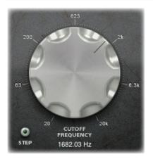
The CUTOFF frequency dial is the primary control on the Creative Filter. At the full counter-clockwise position, it sets the filter to cutoff at 20Hz. The full clockwise position sets it to a 20KHz cutoff.
